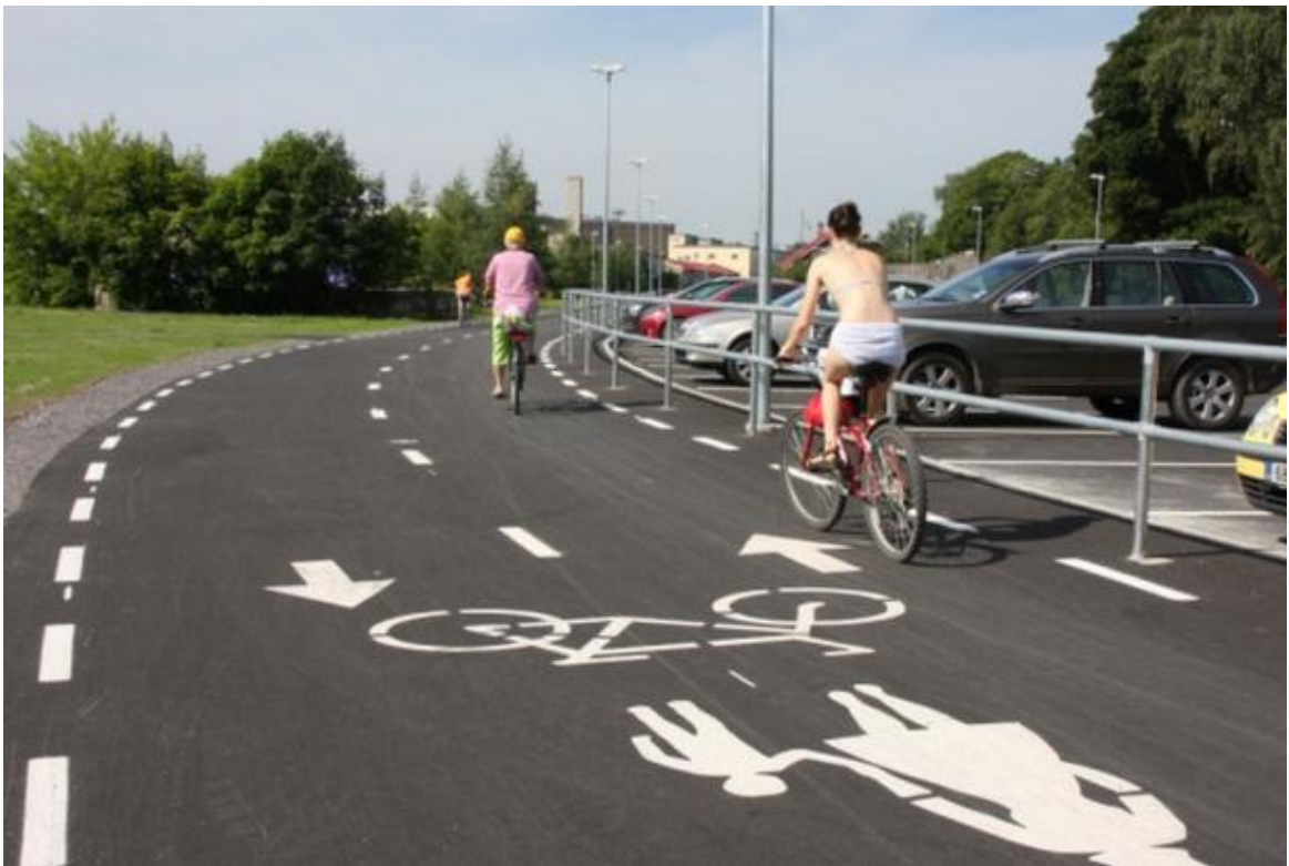
High quality cycle track outskirts of Tallinn, provided by the car parking on the right (Source: Delfi, 2014).
