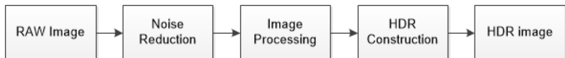
Figure 3.1: The steps that the algorithm takes to achieve the HDR noise reduction.
