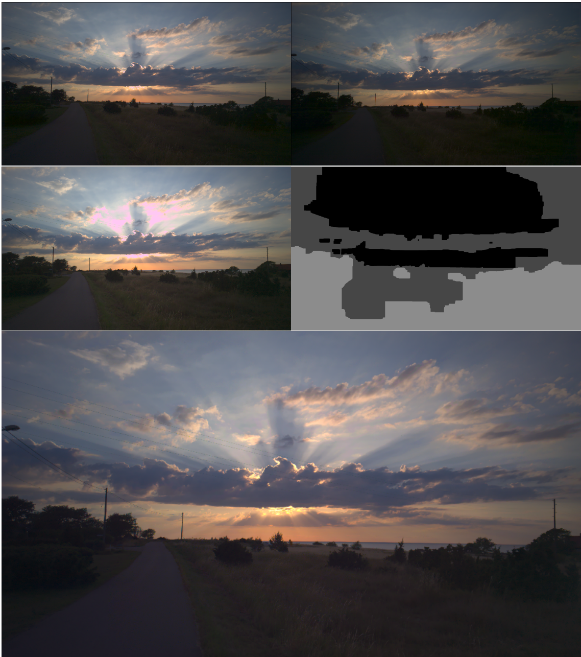
Figure 4.6: The image showcases the selection of the three noise reduced and processed images to make the HDR image. The Top left shows the processed 0EV image. Top right shows the processed -1EV image. Middle left shows the processed +1EV image. Middle right shows the selection corresponding to the \alpha - expansion map, see 3.4.1. The bottom image shows the final HDR image result.
