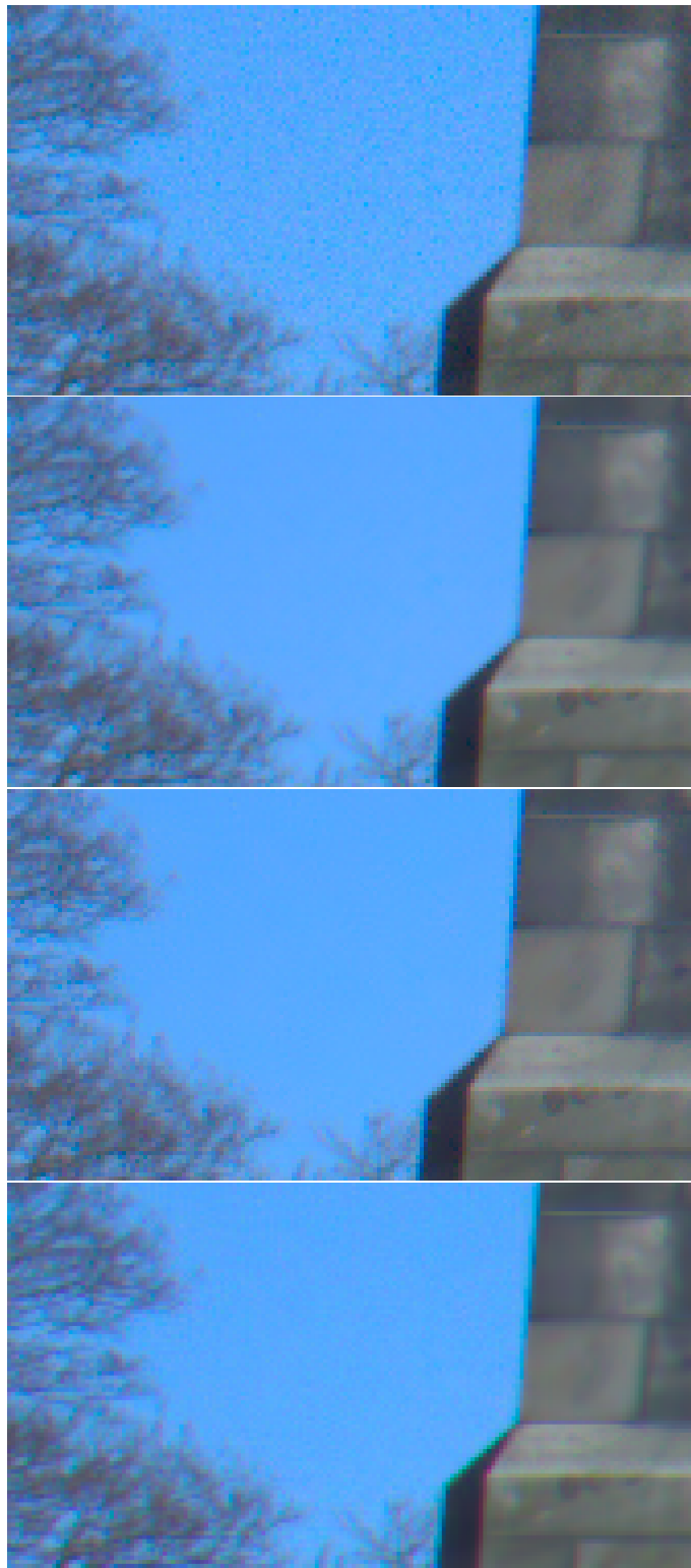
Figure 4.2: Noise reduction comparison for a high noise image. Top is the noisy image, upper middle is the NLM3D algorithm, Bottom middle is the NLM1D algorithm and at the bottom is the BM3D with a constant noise level.
