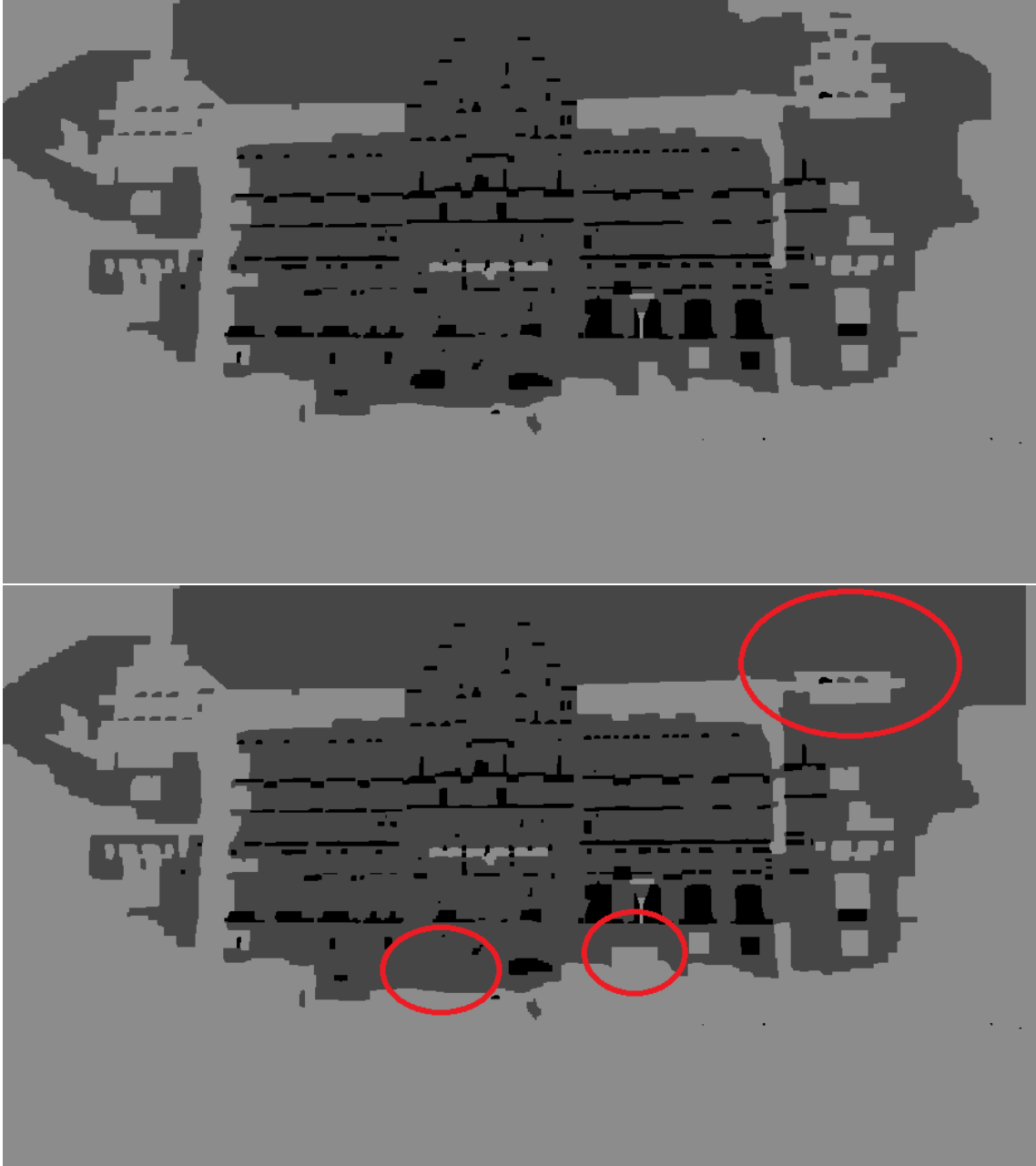
Figure 4.12: Image showing a map which introduces ghosting (top) and an image showing the manually edited map to prevent these artifacts (red circles) in bottom picture.
