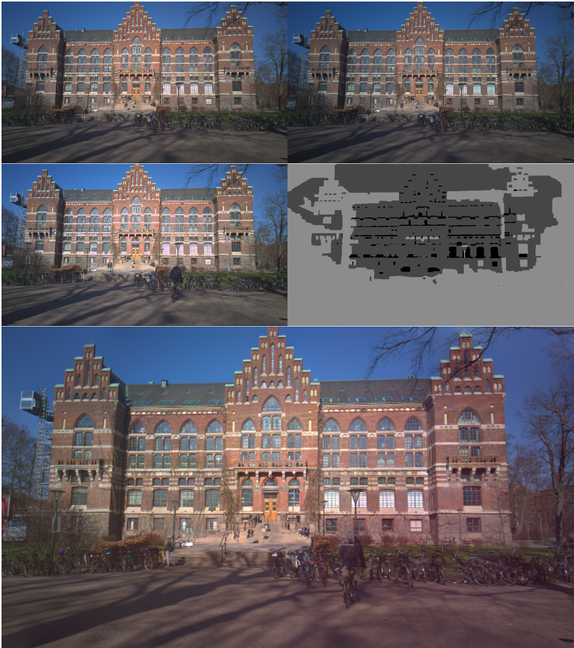
Figure 4.8: The image showcases the selection of the three noise reduced and processed images to make the HDR image. The Top left shows the processed 0EV image. Top right shows the processed -1EV image. Middle left shows the processed +1EV image. Middle right shows the selection corresponding to the \alpha -expansion map. The bottom image shows the final HDR image result.
