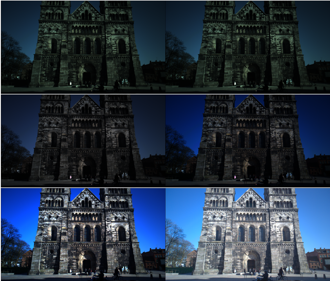
Figure 4.5: Images showing the workflow according to the image processing seen in 3.4, Top right shows the raw image from the sensor, the only processing done is that of noise reduction. Top right shows the Linearized data, i.e the darkest value is 0 and the brightest one is 1. Middle left image shows the image after white balance on each respective channel has been performed. Middle right image shows the image after the color has been corrected to the "right" space, i.e more suitable to be viewed from a computer screen. Bottom left image shows the image after brightness correction has been made. Bottom right shows the final image after another correction has been made in form of gamma correction.
