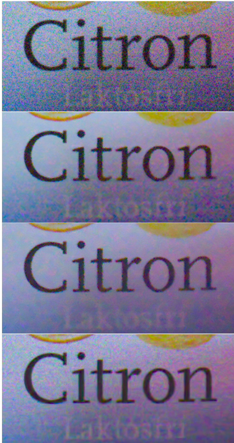
Figure 4.3: Noise reduction comparison for a high noise image. Top is the noisy image, upper middle is the NLM3D algorithm, Bottom middle is the NLM1D algorithm and at the bottom is the BM3D with a constant noise level.
