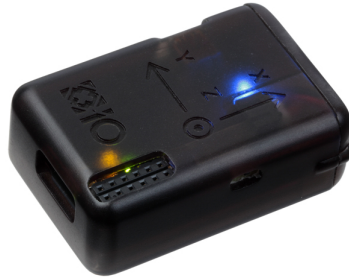
Figure 3.3: Inertial Measurement Unit (IMU) from x-io Technologies, from [46].
