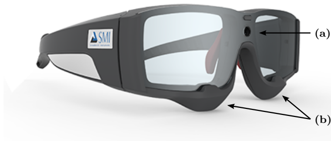
Figure 3.2: SMI eye-tracking glasses. Letters indicate the locations of a) the scene camera and b) the eye cameras, from [44].
