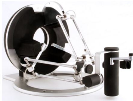
Figure 3.3 Omega 7 haptic device, copyright of ForceDimension
