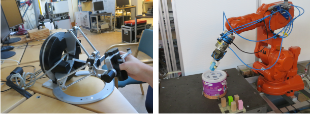
Fig. 5. The test setup used to evaluate the quality of the bilateral teleoperation. The left image show the Omega.7 haptic device and the right image show the ABB IRB 140 industrial robot.
