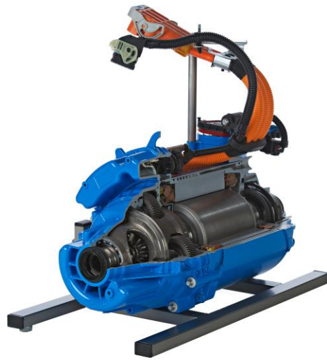
Figure 2.7-1 ERAD cross section cut. Courtesy of Magna Powertrain.
