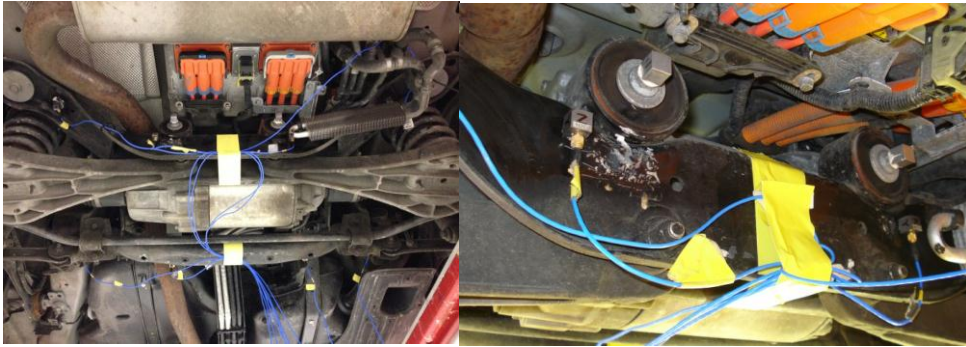
Figure 3.1-2 Rear suspension with accelerometers glued at arbitrary points and aluminum bosses glued to mounting points
