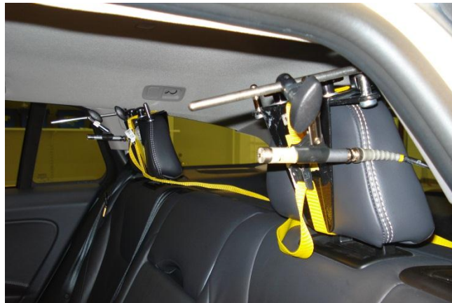
Figure 3.1-1 Microphones at outer ear position in V60 rear seat
