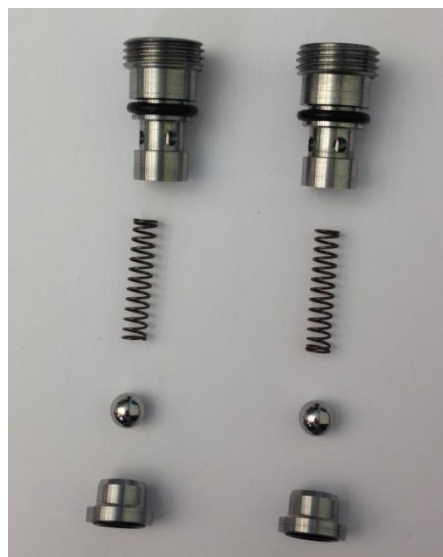
Figure 7.3 The two De-air interval valve prototypes before assembling.
