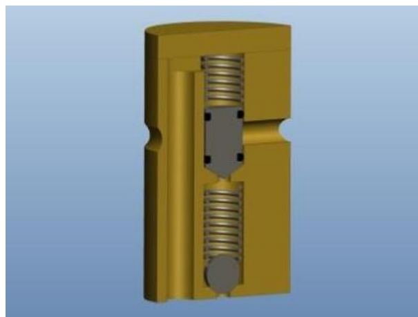
Figure 5.13 Concept 17 – Valve that opens at pressure drop.
