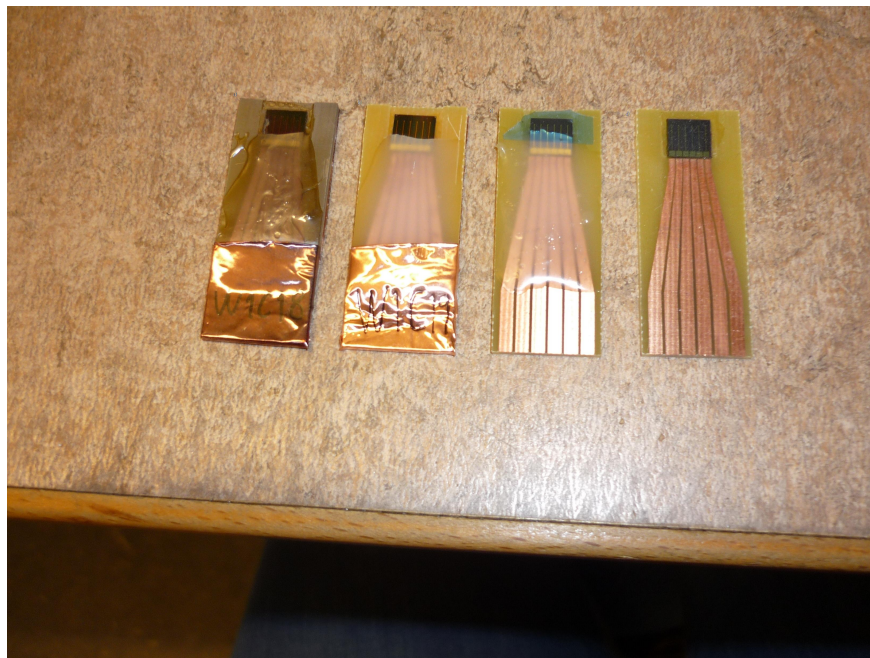
Figure 10: Four samples in different states. From the left: a sputtered and copper taped sample with silicone, a copper taped sample with silicone, a sample with silicone (the blue plastic is protecting the electrodes from contamination) and an untreated sample.
