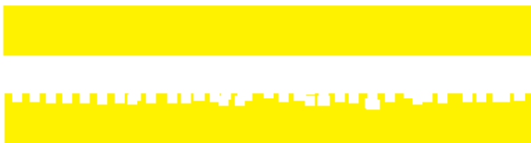
Figure 2: Schematic drawing of planar gold, above, compared to nanoporous gold, below, of the same geometric size. It can easily be seen that the real surface area is significantly larger for the porous gold than for the planar gold.
