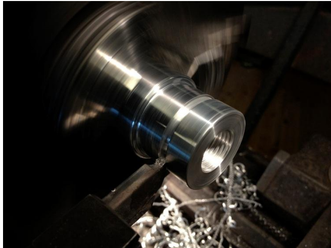
EXHIBIT 5-10 Picture showing top-ring cut off.
