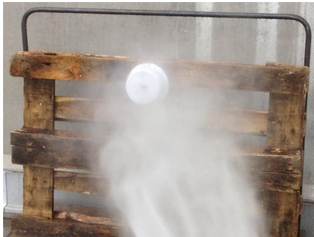
EXHIBIT 6-4 Picture is showing water test rig sprayed with water jet.
