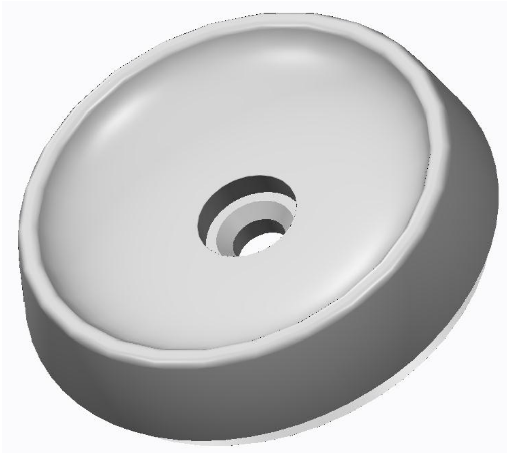
EXHIBIT 4-11 The top-lid showing a dish-like design with a middle hole for the microphone.
