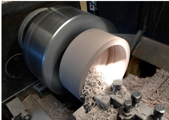
EXHIBIT 5-6 Picture of hollowing out the bottom housing.
