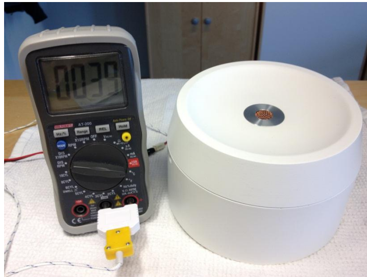
EXHIBIT 6-5 Picture is showing heat test set up including temperature.
