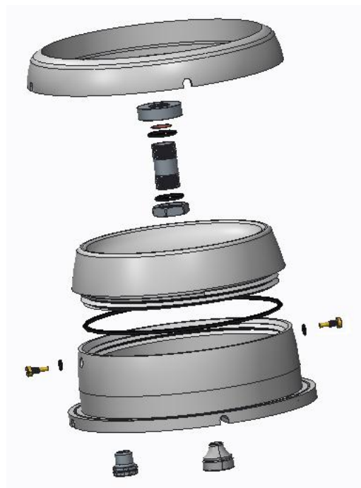
EXHIBIT 5-13 Picture showing all parts included in the housing.
