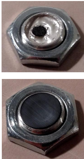
EXHIBIT 5-25 Picture, top-left embedment of microphone in silver epoxy, low-left tube orifice attached with Gore ® membrane, right showing microphone assembled.
