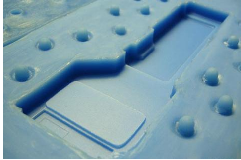
EXHIBIT 5-2 Picture showing rubber mold for resins casting
