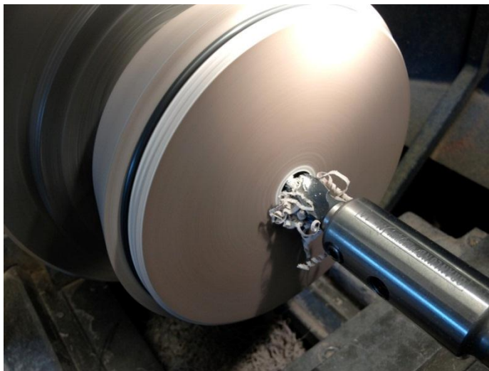
EXHIBIT 5-7 Picture of top lid drilled for microphone tube.
