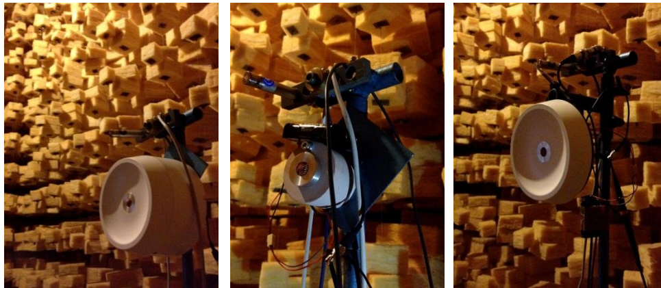
EXHIBIT 6-3 Picture is showing the different test rigs. From left: complete housing, middle: microphone only (apart from housing), right picture: top lid only including microphone. Reference microphone is seen in top left of pole.
