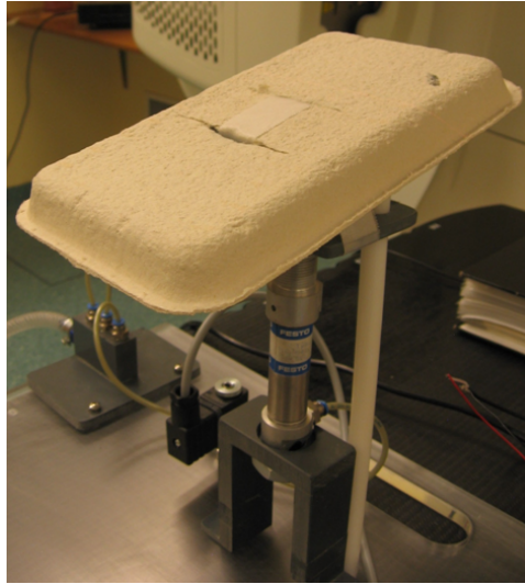
Figure 11: The cardboard assembled on the pneumatic piston.
