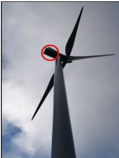
Figure 3. The wind turbine with the acoustic detector D500X. The red circle shows the back of the nacelle, from where a microphone connected to the acoustic detector D500X is hanging out through an opening underneath the nacelle.
