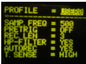
Figure 4. Profile settings for the acoustic detector D500X. SAMP. FREQ is the sampling frequency. PRETRIG will store audio from before the trigger. REC. LEN is the length of the recording, in seconds. HP-FILTER is a high-pass filter that only let signals above 20 kHz to get through. AUTOREC is the automatic recording mode. T. SENSE determines the duration of the signal at which the recording will be triggered.
