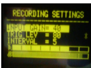
Figure 5. Recording settings for the acoustic detector D500X. INPUT GAIN is the gain added to the recording. The TRIG LEV is the trigger level, the level at which recording starts. INTERVAL is the minimum time between recordings, in seconds.
