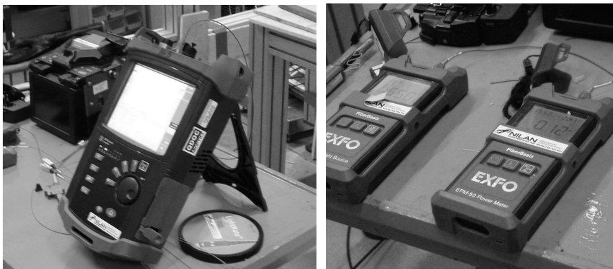
Figure 5 - In the left picture is the OTDR device and in the right picture is the OPM devices.
