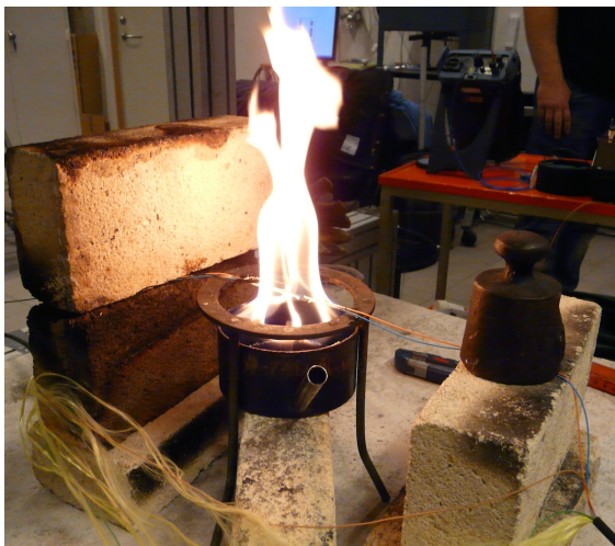
Free burning experiment, standard setup (left picture), cable bundle setup (right picture)
