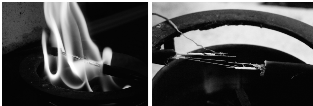
Figure 12 – The left picture is taken during the free burning, whole cable experiment (MM) and the right is taken after it ended. The broken fibers are clearly visible in the right picture.
