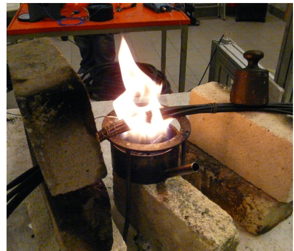
Free burning experiment, standard setup (left picture), cable bundle setup (right picture)
