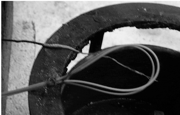
Figure 11 - Free burning experiment, bending radius setup (steel wire).
