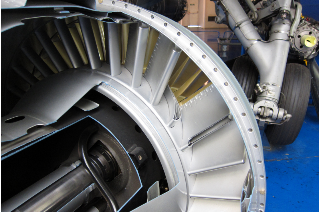
Figure 1: The inlet guide vanes of an Atar turbojet. Air flows from the viewer towards the background of the photo [2].
