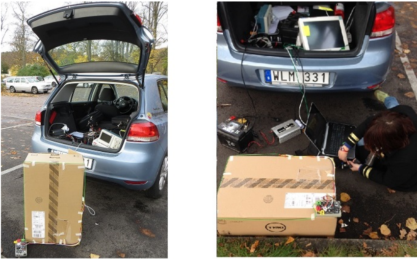
Figure 13: The setup for the measurements in Göteborg. The wires were taped to a box, which lay down on the ground or was placed standing. Inside the car the monitor is seen. In the right hand picture a trailer battery and a converter is seen, which were used to power the monitor.
