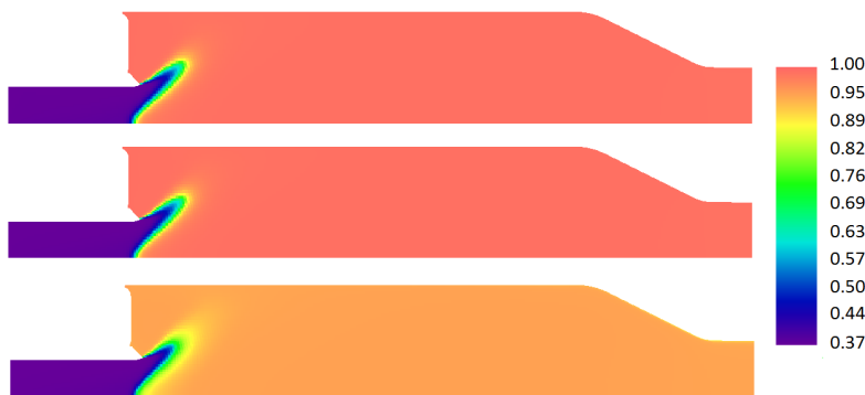
Figure 16: Calculated temperature fields in the Siemens burner rig. For confidentiality reasons the plot is stretched and a relative scale is used where all values are compared to the maximum temperature in the 166 species homogeneous reactor simulation. Above: homogeneous reactors using the 28 species mechanism. Middle: homogeneous reactors using the 166 species mechanism. Bottom: CMC using the 166 species mechanism.
