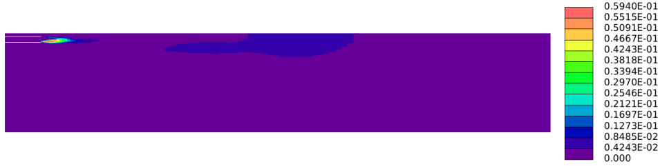
Figure 7: Root mean square (RMS) fluctuations from time averaged mixture fraction over 0.01 s. Calculated for the Sandia D homogeneous reactor 163 species baseline case.
