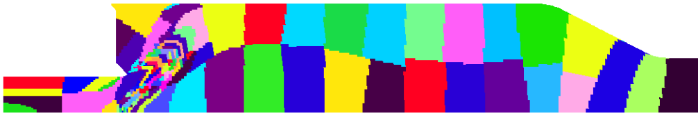
Figure 18: Baseline reactor network for Siemens burner rig constructed with the PCA method from computational fluid dynamics simulations based on the 28 species mechanism. All cells belonging to the same zone have the same color. Some disconnected zones also have the same color, this does not mean that they are the same zone. Every zone is a geometrically connected set of cells.
