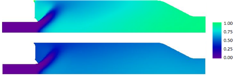
Figure 17: NO mass fraction fields in the Siemens burner rig calculated with the 166 species homogeneous reactor model. Above with adiabatic walls and below with fixed temperature walls. For confidentiality reasons the plot is stretched and a relative scale is used where all values are compared to the value at the outlet from the simulation with adiabatic walls.
