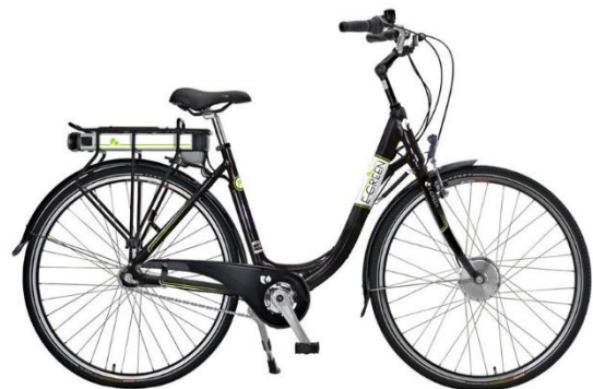
Figure 3. EPAC with engine in front wheel hub and battery under carrier. Copyright Merida Sweden AB.
