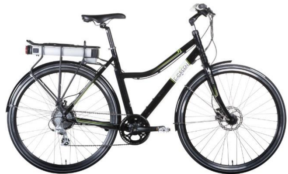
Figure 2. EPAC with motor in back hub and battery under carrier. Copyright Merida Sweden AB.
