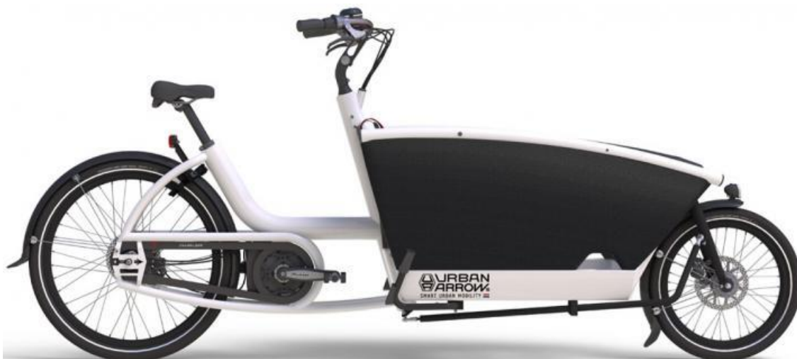
Figure 19. The Urban Arrow, model Family. This e-bike still meets the demands of an EPAC but could gain from a more powerful engine since it is possible to transport two children in this bicycle.
