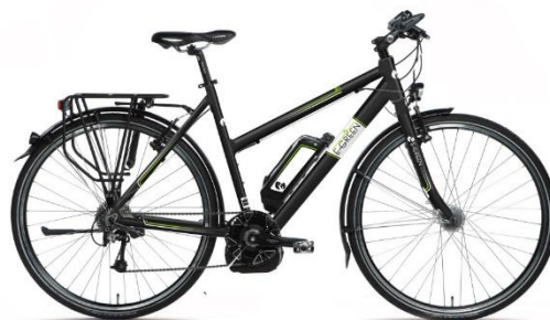
Figure 4. EPAC with engine in crankset and battery on frame. Copyright Merida Sweden AB.
