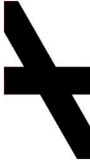
Figure 4.8: Smallest possible slab element which can correctly represent the entire weave electromagnetically.
