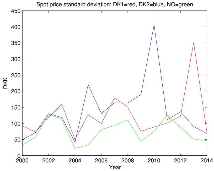
Figure 4.10: Annual standard deviations of spot price for three Nord Pool bidding areas: DK1 (red), DK2 (blue) and NO2 (black). The deviation in spot price is notably higher in the Danish regions.
