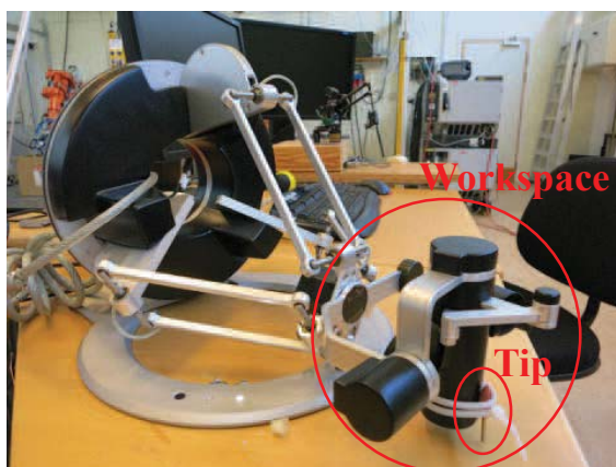
Figure 3.1 Robot (Omega7) used in the experiments.
