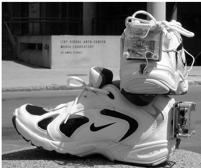
Figure 7: Piezoelectric-powered shoes with its electronics mounted 17
