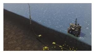
Figure 3. Floating wind power can be used to power the water injection pump raising the pressure of the oil reservoir and thereby increasing the potential oil extraction. Such an application could dramatically reduce the  $CO_2$  emissions of offshore oil & gas activities on the Norwegian continental shelf.
