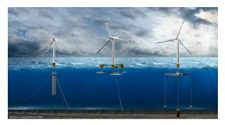
Figure 1. Three different floating wind power concepts. From left to right: The Spar Buoy, the Semi-Submersible and the Tension Leg Platform (TLP). The main difference is the way stability is achieved for each of the platforms. The TLP is mooring stabilized, the Spar is ballast stabilized and the semi-sub is buoyancy stabilized
