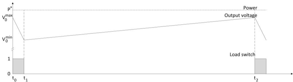
Figure 4.7: Voltage ripple for a perfect period on the DC-output.
