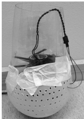
Figure 5.7 A prototype made from the sketch. Used to examine the size of the holes to provide a good airflow to the fan.
