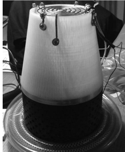
Figure 5.11 The lampshade holder and the fan cover are attached to the design by screws.
