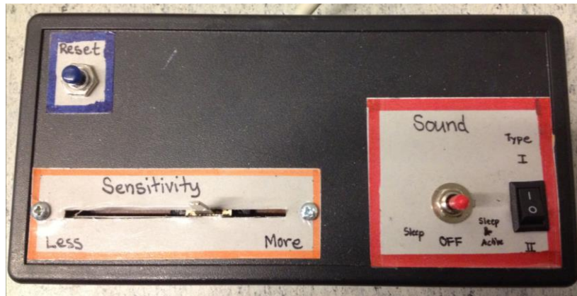
Figure 5.29 With the control box the GlowNado can be reset, the sensitivity of the capacitive sensor can be adjusted and the different settings for the sound can be chosen.
