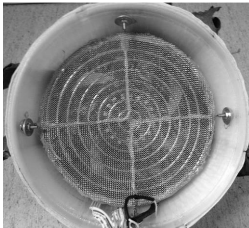
Figure 5.12 Seen from the inside. The fan is attached to a fan cover at the bottom of the upper part of the design.
