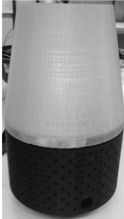
Figure 5.9 The final 3D printed version. The lower part is black to avoid attraction and the upper part is transparent white to attract the user to the wind.
