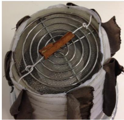
Figure 5.25 A cinnamon roll was placed on the fan cover, the fan helps spread the scent.
