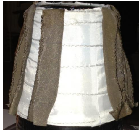
Figure 5.14 Conductive thread was sewn in a spiral and seven stripes of brown conductive fabric were added to work as a sensing material.
