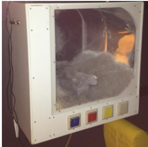
Figure 4.1 The user can switch colors with the buttons, and turn on and off the fan. The feathers inside gives a visual effect of the wind, the fan is creating.
