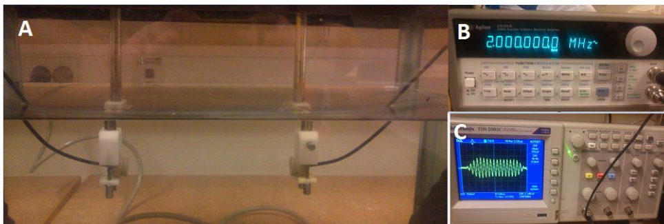
Figure 34 A) Aquarium with two 2 MHz transducers (circular), B) Function generator connected to the right transducer, C) Oscilloscope connected to the left transducer
