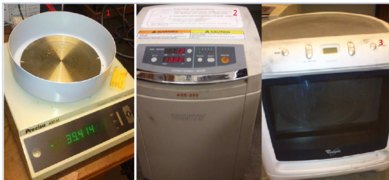
Figure 26 Scales, centrifuge and microwave oven used in the process of making an agar phantom
