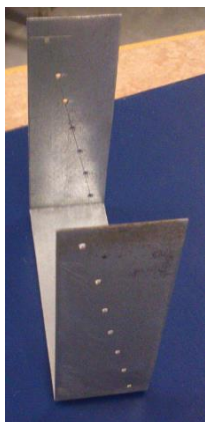
Figure 30 The testing frame with the larger lateral distance between the top and bottom hole
