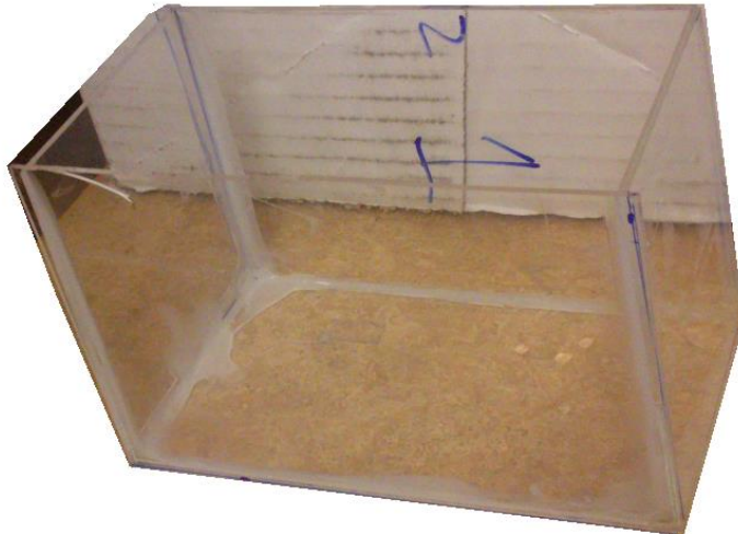
Figure 36 Empty phantom container made from 3mm PMMA
