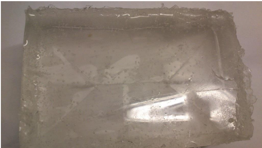
Figure 32 Example of candle gel with bubbles
