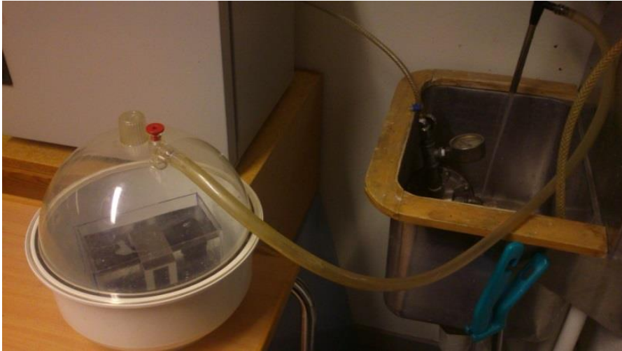
Figure 33 The water driven vacuum pump system
