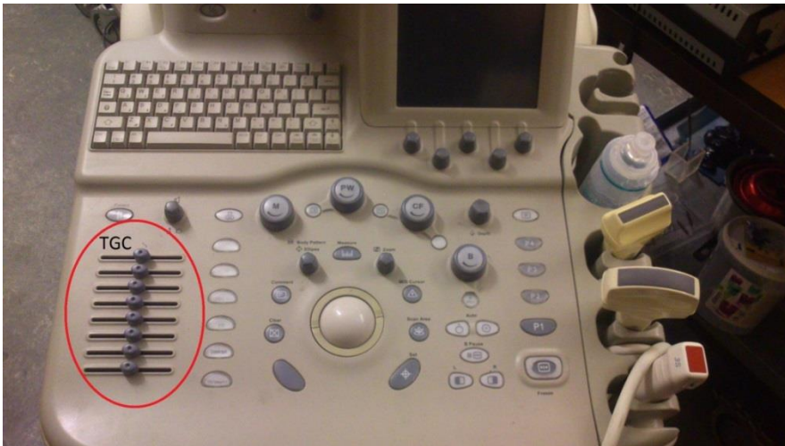
Figure 8 User interface of a typical ultrasound machine, circled in red is the TGC interface
