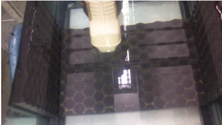
Figure 28 Transducer and dampening pads in the water tank
