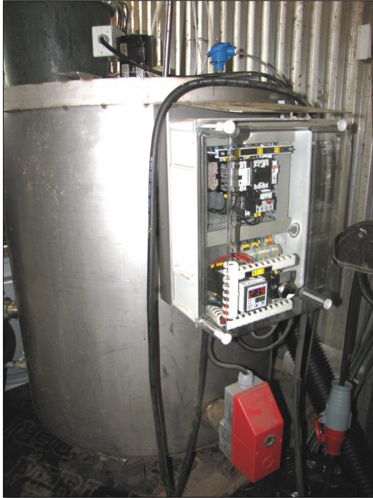
Figure 3-7. Pretreatment reactor used in full-scale experiment (Volume = 170 liters).
