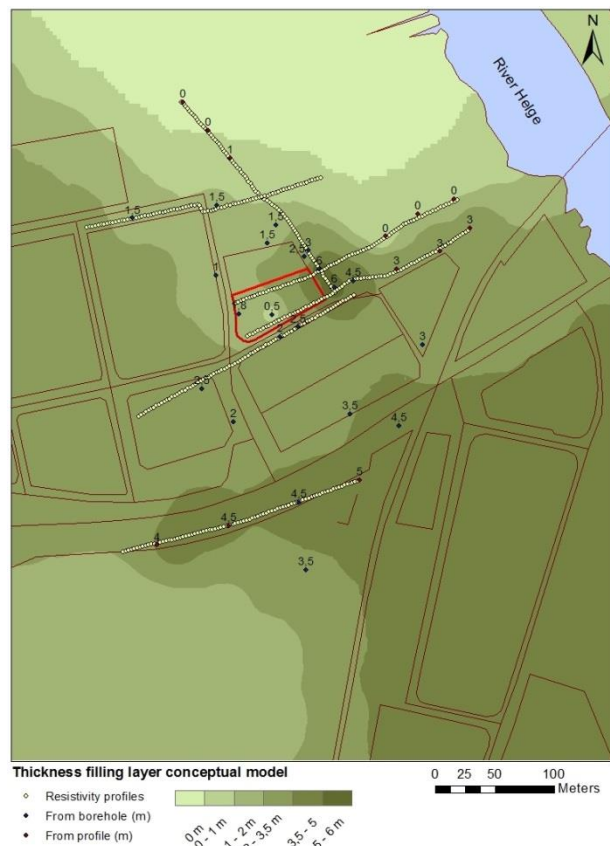
Figure 38. Horizontal overview of the thickness of the fill layer in geological model 2 and 3. The dark blue points show the location of the boreholes and attached number the observed thickness. The red points mark additional information regarding the layer thickness retrieved from the resistivity profiles. The red polygon shows the location of Färgaren 3
