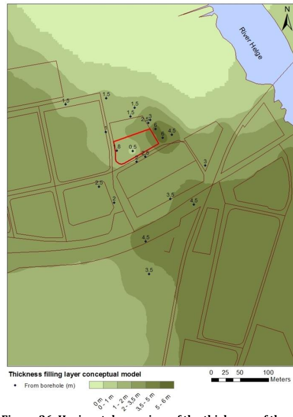
Figure 36. Horizontal overview of the thickness of the fill layer in geological model 1. The dark blue points show the location of the boreholes and attached number the observed thickness. The red polygon shows the location of Färgaren 3
