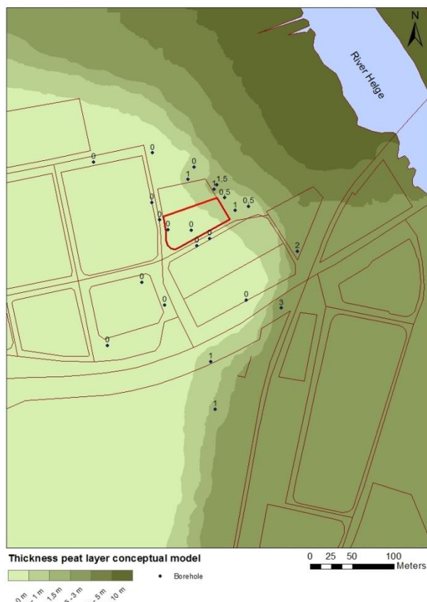
Figure 41. Horizontal overview of the thickness of the peat layer for all three models. The dark blue points show the location of the boreholes and attached number the observed thickness. The red polygon shows the location of Färgaren 3
