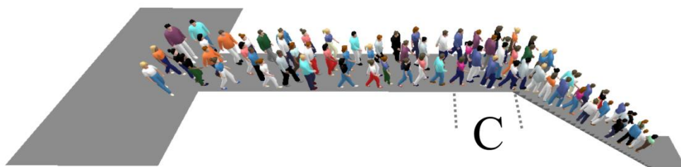
Figure 31. Congestion in front of the stair (the area denoted C) after 50 s.
