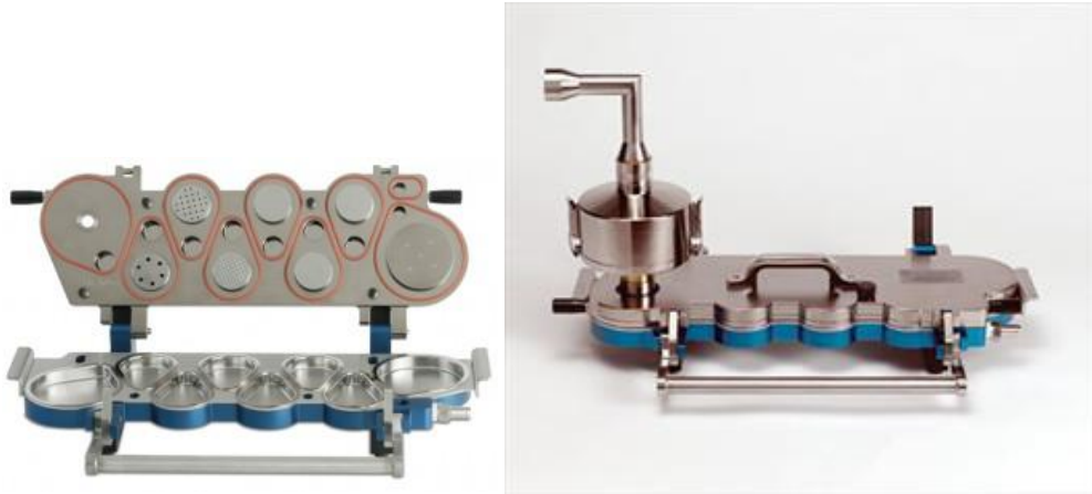
Figure 1.3 : The image to the left displays an open NGI. The image to the right displays an NGI connected to a United States Pharmacopeia (USP) induction port and a pre-separator, mimicking the upper airways of the lungs. Typically a DPI is connected the inlet of the NGI, in which the powder is drawn from. In this work, a prototype device, described in chapter 3, was used. The airflow is lead from left to right, and the small cavities seen in the left figure fractionates the aerosol by impaction. [12, 13]
