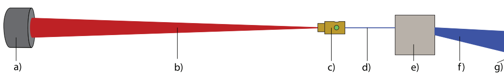
Figure 4.3: Sketch of the experimental setup. a) Parabolic mirror, b) laser beam, c) gas cell, d) electron beam, e) dipole magnet, f) dispersed electron beam, g) scintillating screen. The laser pulse is focused into the gas cell. Laser wakefield acceleration of electrons takes place in the cell. The electrons exit from the gas cell to the right traveling into a spectrometer.
