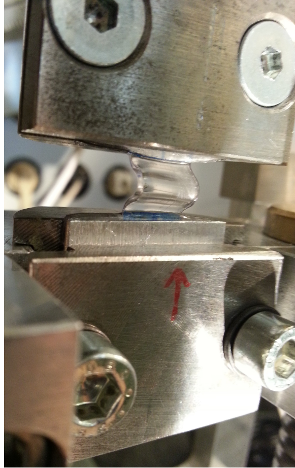
Figure 5.1: Photo showing how the sample buckles when it is clamped
