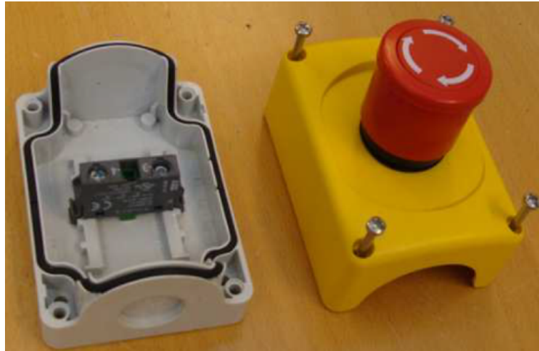
Figure 3.1: Picture of the button used in the case study. The screws are not part of the case study assembly
