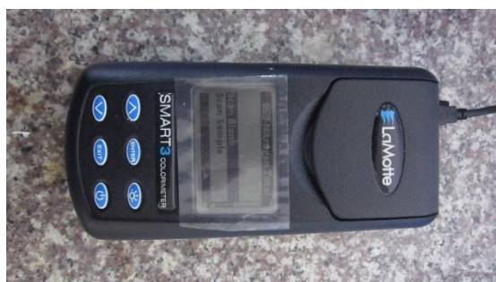
Figure 4.6. Photo of the SMART 3 colorimeter.
