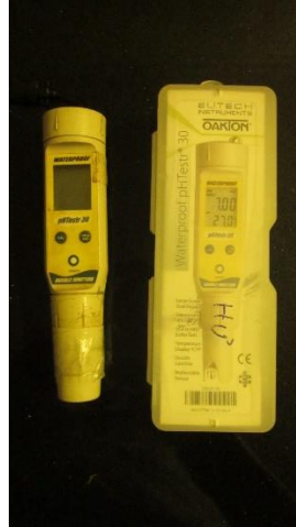
Figure 4.4. Photo of the pHTestr 30 from Eutech instruments used for pH measurement at the factory.
