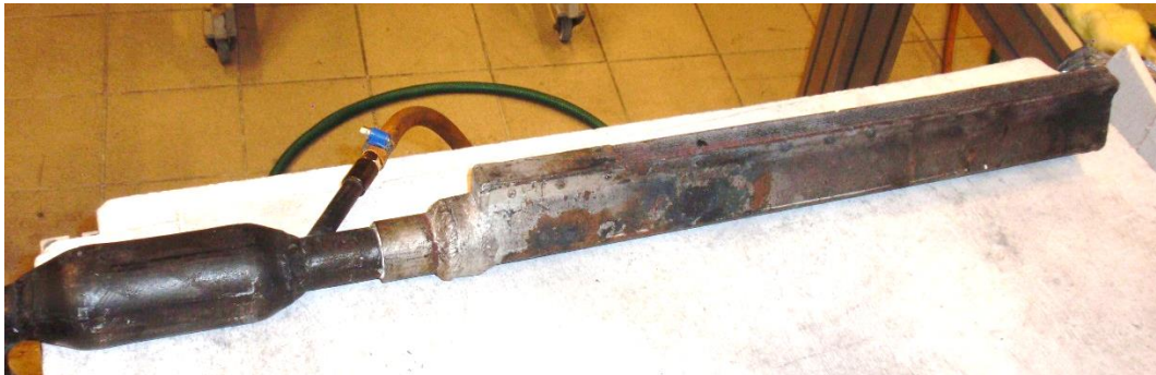
Figure 8. Gas line burner
