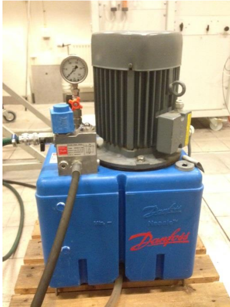
Figure A-1 . Danfoss Power Pack PPH 6.3 with a piston pump used throughout the study
