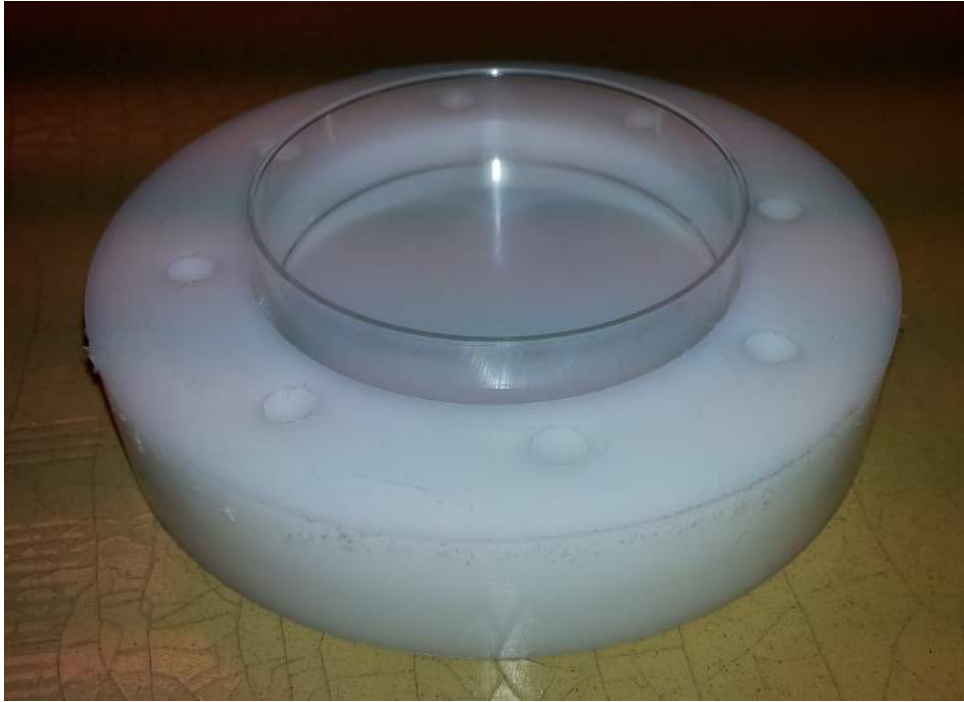
Figure 32: Bottom piece of the device holder. A cell culture dish is submerged into the milled cavity. Eight screw holes are evenly milled around the cell culture dish.
