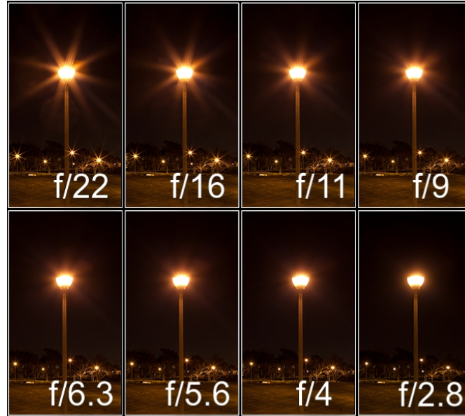
Figure 2.3: Aperture diffraction occurs at the entrance pupil of the camera, and is seen as the star-shaped light around the sources. The shape varies depending on what aperture is used. In (2.4), it is assumed that the aperture is circular, which results in a circular aperture diffraction. The extent of the aperture diffraction is connected to the focal length of the camera. Image source: www.slrlounge.com/school/diffraction-aperture-and-starburst-effects .
