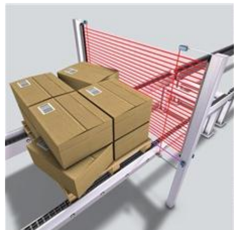
Figure 11. Pallet overhangs. (SICK, 2014)
