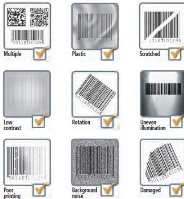
Figure 9. Readable barcodes by Cognex's solution (Cognex, 2013)
