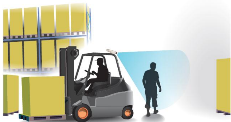
Figure 20. Illustration of the human detection for forklift application (Axis, 2015f)
