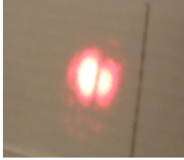
Figure 12: The probe beam imaged on a piece of cardboard just after the beamsplitter. A large interference fringe owing to the etalon-effect of the beamsplitter is visible, splitting the beam.
