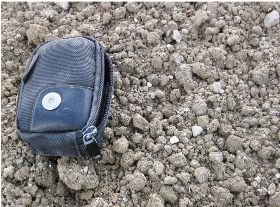
Figure 4.4 The appearance of the mixed modified clay till before compaction occurs.
