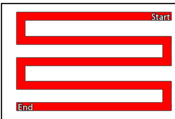
Fig 15. Measurement methodology used in this study for the slingram measurements, by moving from start to end accord-
