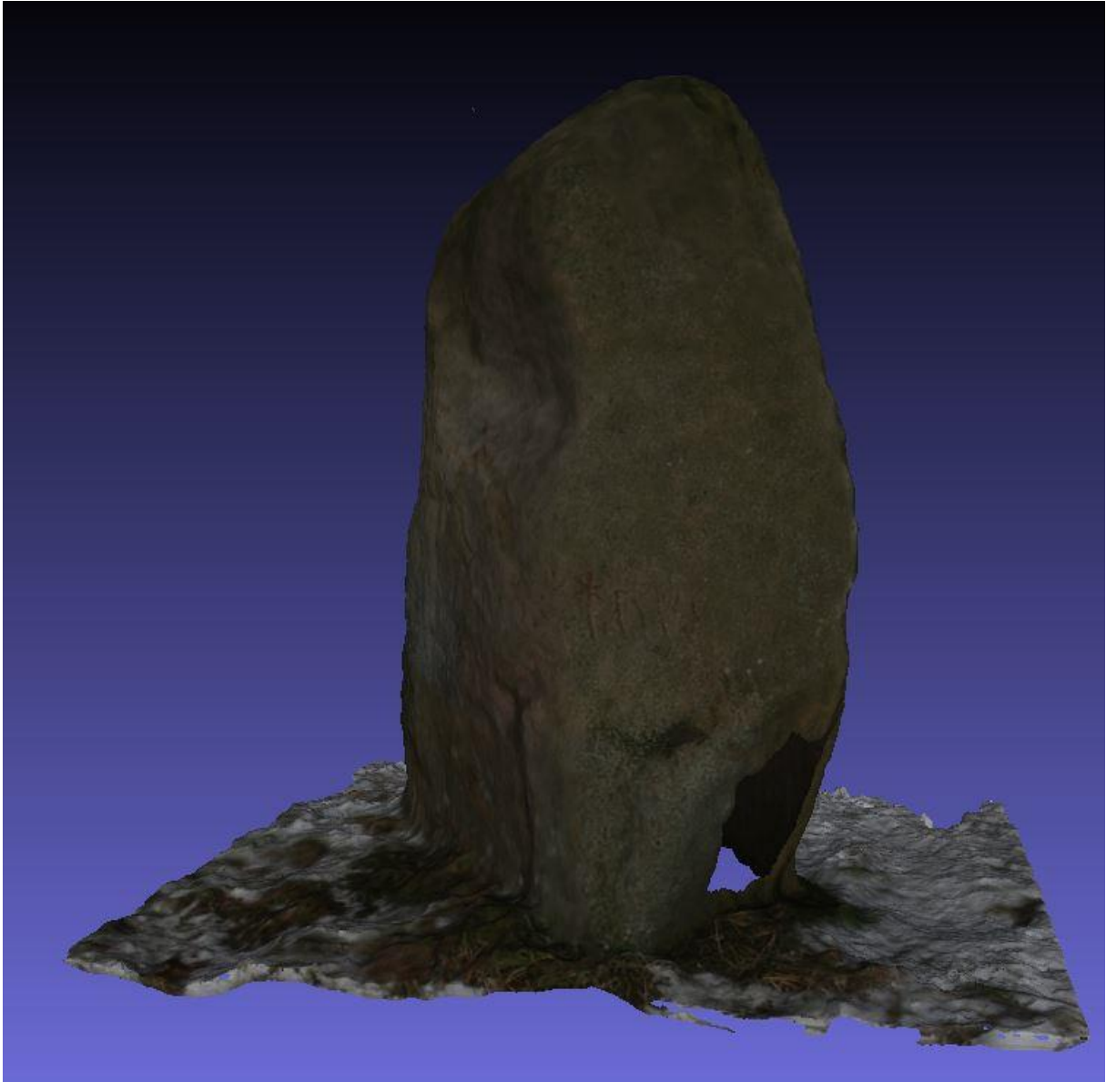
Figure 23. A visualization of the side of the first model, with texture created in Agisoft Photoscan, imported to Meshlab.
