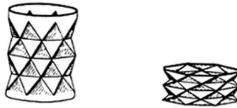
Figure 40: Collapsing mode of the can with circumferential polyhedral wall (Ishinabe et al., 1992)
