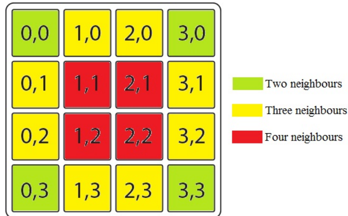
Figure 2.7: The picture illustrates how many neighbours each core has in a 4x4 grid
