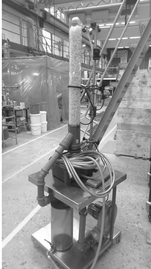
Figure 3.1. The equipment that's used in the experimental part. At the top, water is sprayed out and distributed into the column. The fan, seen on the lower level, blows air through the tank and up into the column where it's pushed through and out on the top.
