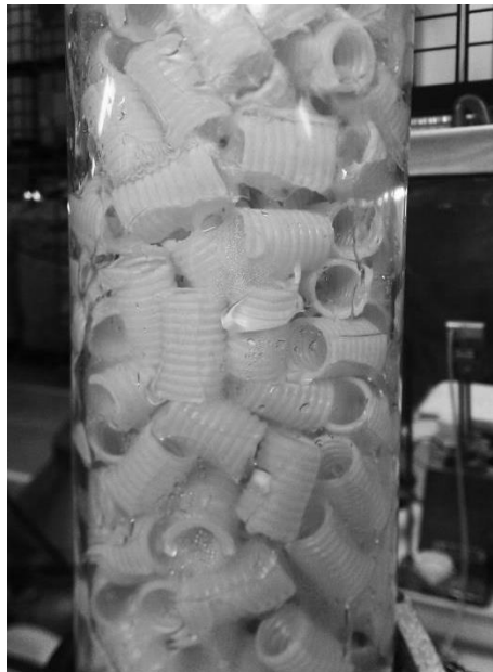
Figure 3.3. This is what the packing looks like. The distribution of the water phase can also be seen since the column is active. Note that a lot of the water is located at the edges of the column.
