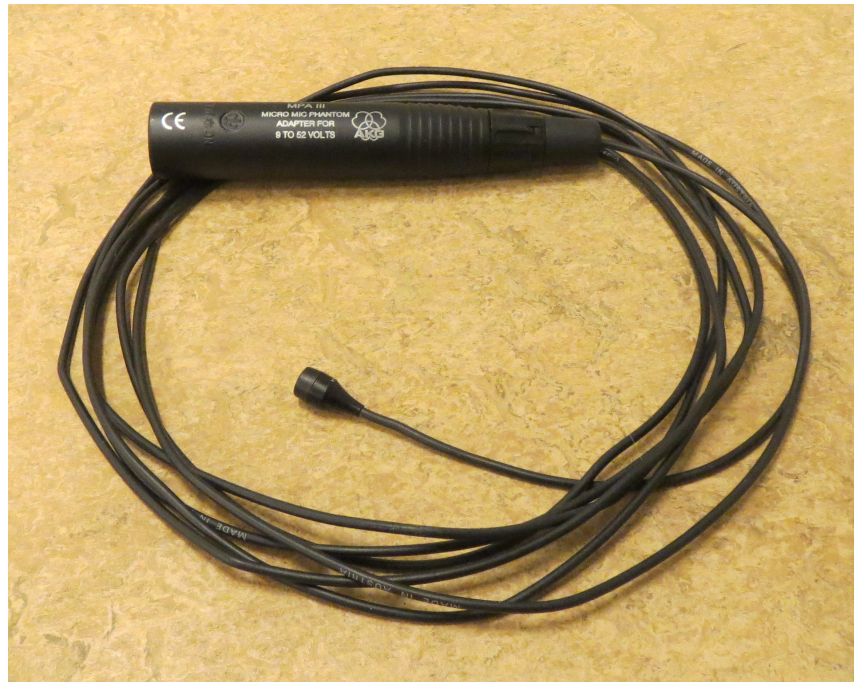
Figure 2.5: AKG C417 condenser microphone with AKG MPA III phantom adapter
