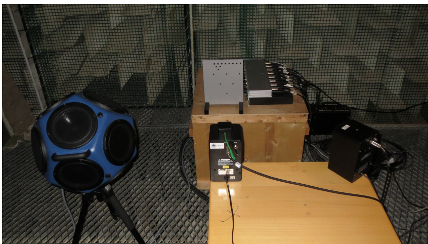
Figure 2.12: Configuration of the equipment inside the anechoic chamber
