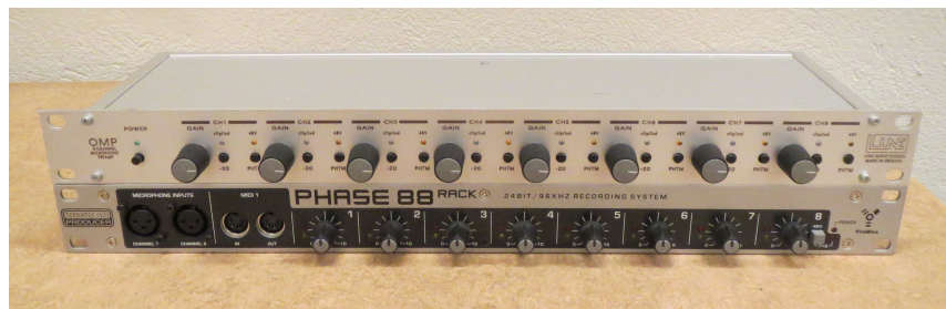
Figure 2.6: 8 channel microphone preamplifier from Line Audio Design and Terratec PHASE 88 Rack FW audio interface
