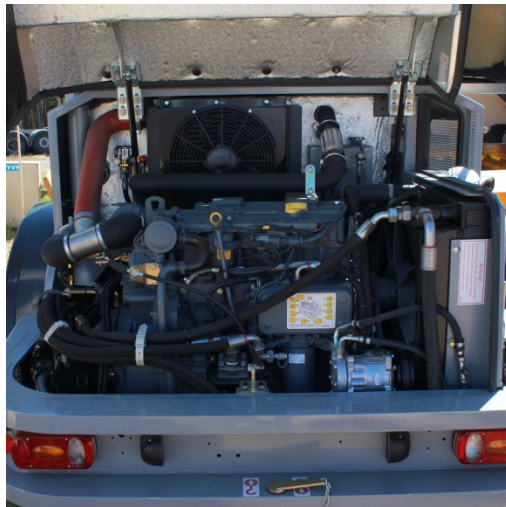
Figure 2.3 – Engine compartment layout of a small excavator. Courtesy of SP.
