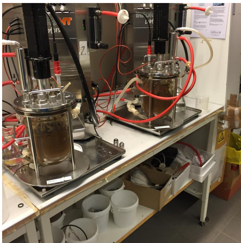
Figure 3.3. 2L laboratory fermenters from Infors AG
