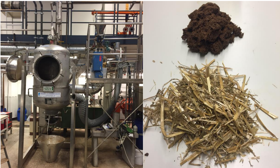
Figure 3.1. Steam explosion unit used for pretreatment and the appearance of wheat straw before and after pretreatment.
