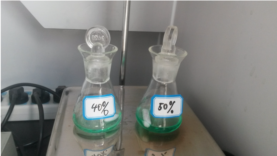
Figure 10 depicts the mixed slurries for the 40- and 50 wt% YSZ-NiO slurries. The green colour originates from the \text{Ni}(\text{NH}_3)_2 crystals.
