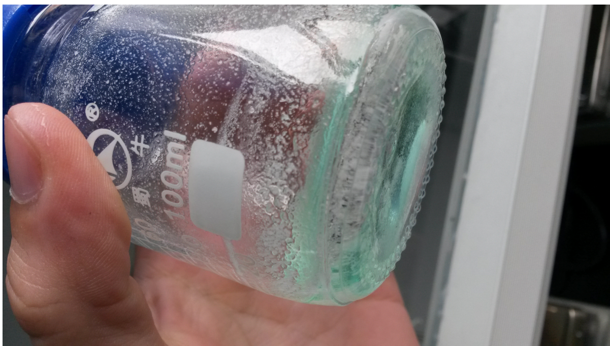
Figure 28 depicts a beaker with rejected slurry due to precipitation. The crystals are shown clearly as white spots on the walls.
