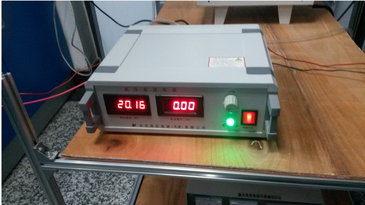
Figure 15 showing the high voltage power supply during operation.
