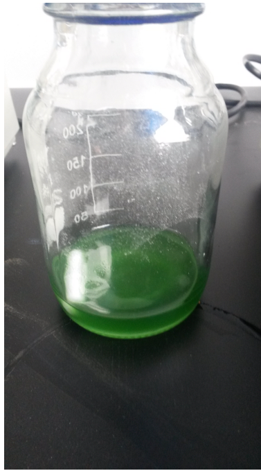
Figure 29 depicts the slurry with too high viscosity before it was put in the syringe for electrospinning
