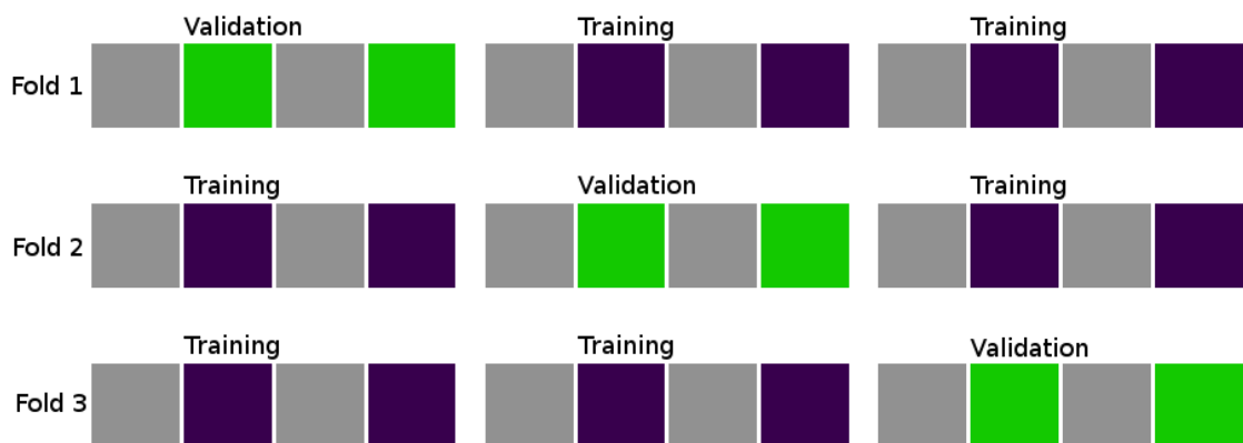
Figure 5.2: A 3 K-fold cross validation example. For each fold two sets are selected as training set and one set is selected as the validation set. All sets take turn acting as the validation set. 10 K-fold is the same, except that it splits the data into 10 folds instead of 3, meaning that for each of the 10 folds 1/10th of the whole data set is used for validation, instead of 1/3rd.
