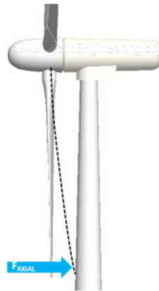
Figure 2.4: Blade bending due to loading [22].
