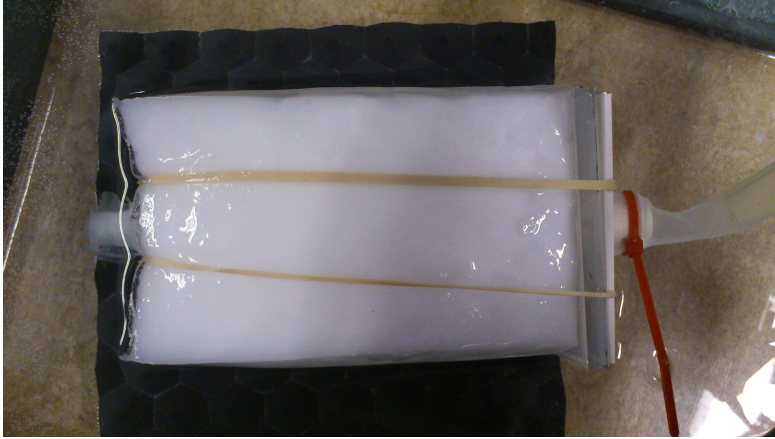
Figure 11: The compound phantom with inlet connection to the right in the image.
