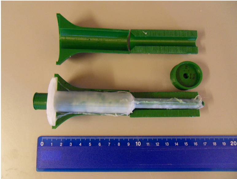
Figure 9: Mold for vessel phantom consisting of six parts. At the top of the image two parts creating the outside contour can be seen. The circular disk to the right forms the base of the mold. Below in the image is a finished phantom with the rod shaping the inner contour still in place. The ruler is graded in cm .
