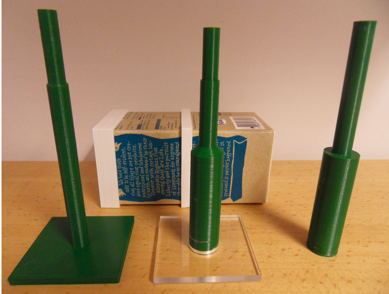
Figure 10: Mold for support structure, in front the rods creating the hole for the three different geometries. In the back the carton with lid and frame (the latter two are white in the image).
